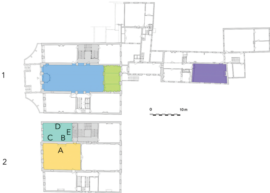
Fig. 16 Plan of the (1) bel-etaage of the 's-Hertogenbosch main town hall complex and second story of the Griffiehuis, and (2) the second story of the main town hall complex, showing the building's internal division after the renovations of 1670 and 1693. Image by Maarten Jansen (Erfgoed 's-Hertogenbosch), based on research by the Municipal Heritage Department of 's-Hertogenbosch (Erfgoed 's-Hertogenbosch). Here indicating the location of the vierschaar (lime green) and trouwzaal (purple), centrale hal (blue), burgemeesterskamer (turquoise), raadzaal (orange), and stairwells (grey), and the current locations of Justice and Concord (A), The right of the four quarters of the Meierij District to appeal before the court of 's-Hertogenbosch (B), The request for admission to the Union (C), Wildman (D) and Two Lions (E).
